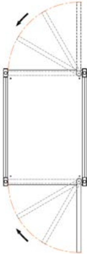
Figure l: Non-hold open configuration
