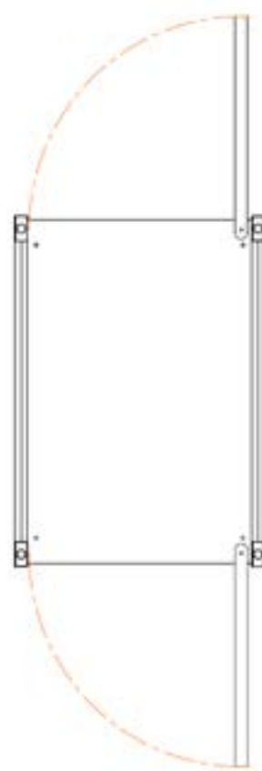
Figure m: Hold open configuration (doors will remain in this position)
