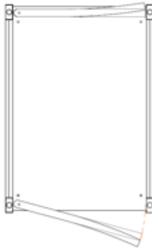
Figure d: Warped doors of an aluminium man-trap
