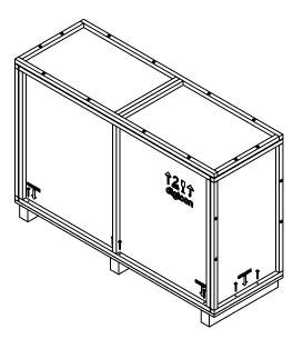
**CAUTION - RISK OF INJURY!:** The packaging, with the equipment inside, is heavy (approximately 140/150kg). To transport it, appropriate lifting equipment is necessary, such as a forklift.
