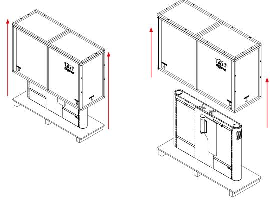
**ATTENTION:** After lifting the box lid vertically, carefully remove the plastic wrap and bubble wrap to ensure the equipment's integrity.
