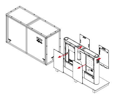
Remove the 8 screws that secure the module to the pallet (use the two 10mm wrenches).
