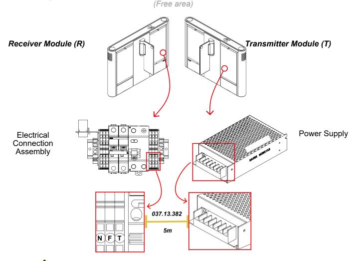
**ATTENTION!** - The cable 037.13.382 is factory-connected to the power supply; it only needs to be connected to the electrical connection assembly of the receiver module.
