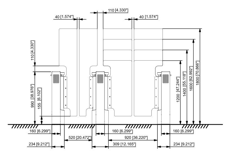
**ATTENTION!** - The dimensions of the dGate modules are illustrated in millimeters and [inches].
