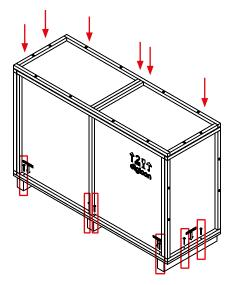
1. Lift the box lid vertically. Ideally, this should be done with two people, lifting it until the lid is above the module.
