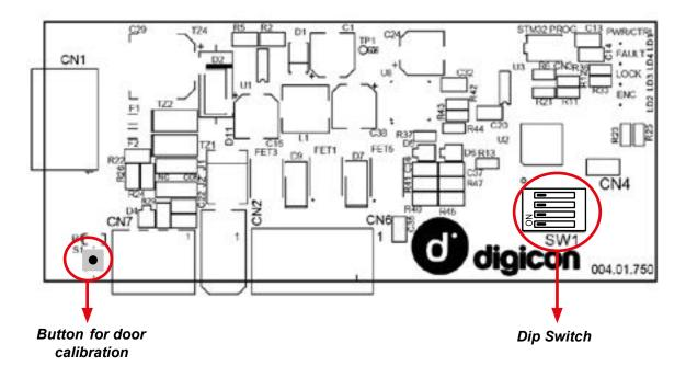
• Press the S1 button on the motor control board for 3 seconds:
