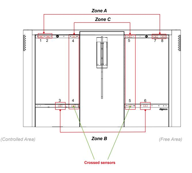
Note: The image above shows a dGate SW, but the sensor positions are the same on the dGate UW.
