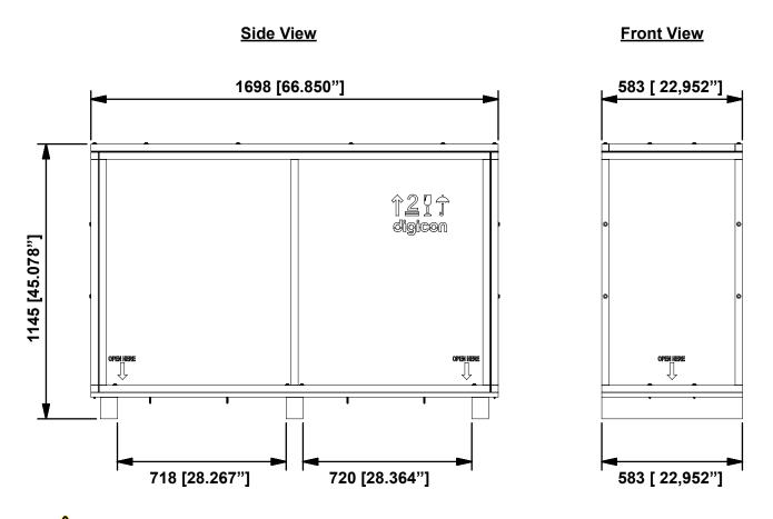
**ATTENTION!** - The packaging dimensions of the dGate modules are illustrated in millimeters and [inches].
