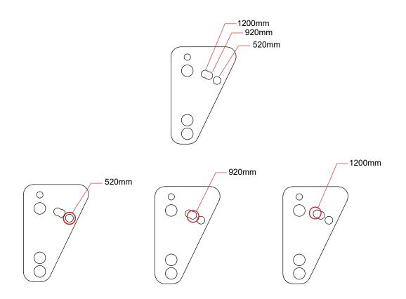
**ATTENTION!** - Since the adjustment for access lanes of 920mm and 1200mm is very close, the adjustment holes on the mount are almost together, without a separation area. Digicon does not recommend using tall doors in access lanes of 1200mm due to the large mass of the doors.
