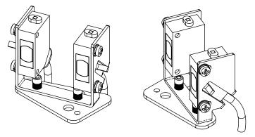
Even in applications where dual transmitters are necessary, only one receiver sensor is used. The goal is to increase the IR transmission field to the single receiver sensor, minimizing trajectory deviations caused by the door's movement.
