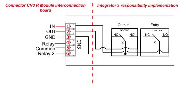
The figure above illustrates an electrical diagram for pass-through activation, where the contacts are made by two external relays to the dGate. This implementation is the responsibility of the integrator (relays not provided).
