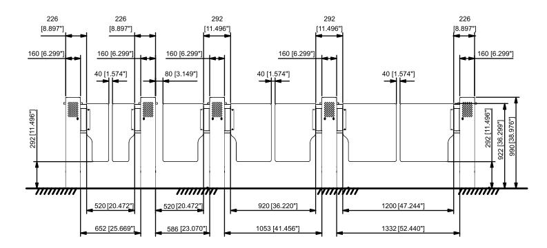
**ATTENTION!** - The dimensions of the dGate modules are illustrated in millimeters and [inches].
