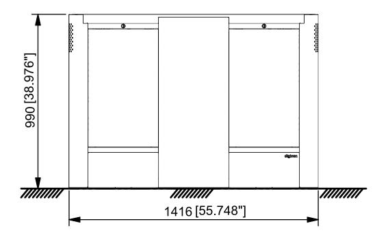
**ATTENTION!** - The dimensions of the dGate modules are illustrated in millimeters and [inches].
